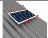
Attach brackets to the roof with roof screws. Seal under the screws and bracket. Run cable under ridge cap and into roof cavity.
